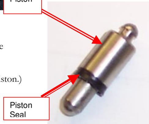
Lubricate Piston Seal with synthetic grease
