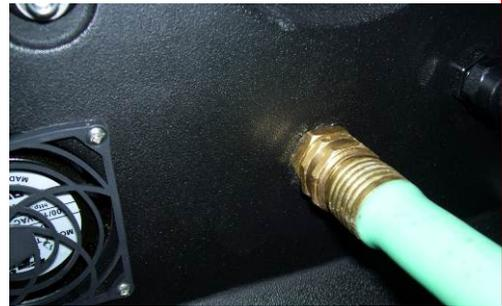
If not using the waste pump-out, the pump-out hose does not need to be connected. When the recovery tank fills during cleaning, the float assembly in the vacuum inlet filter will rise and will automatically shut off the vacuum air flow to prevent the recovery tank from overflowing and waste water from getting into the vacuums.
