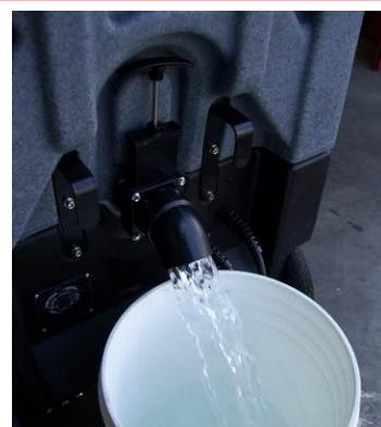
Drain water from Recovery Tank
