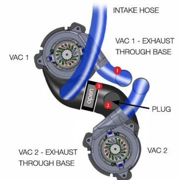
1. Connect Vac 1 exhaust hose to base exhaust port
