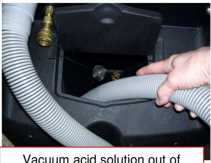
Vacuum acid solution out of Solution Tank
