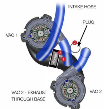
1. Connect Vac 1 exhaust hose to Vac 2 intake port
