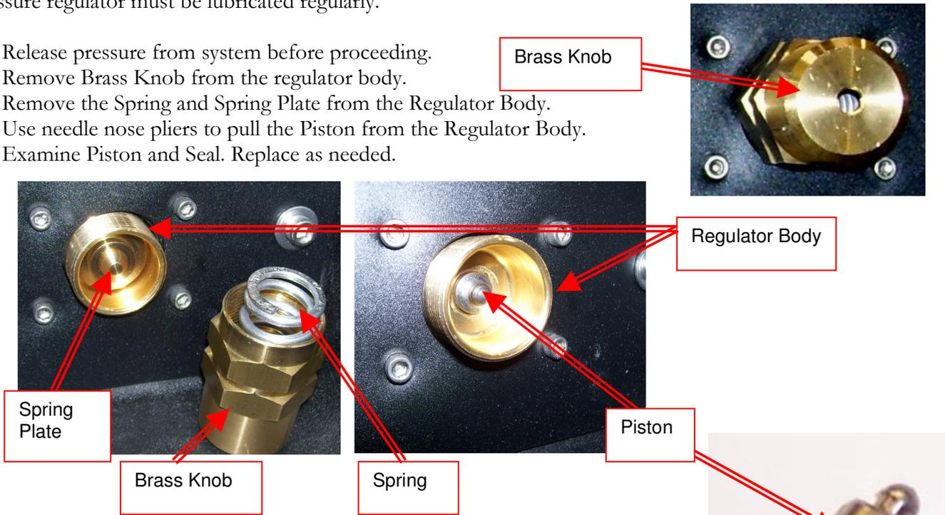
6. Use a synthetic grease with Teflon such as Ultra-Slick or Super-Lube to lubricate the seal on the regulator piston.
